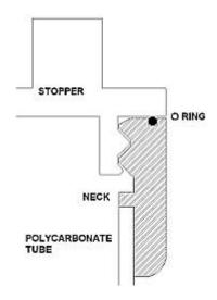
In respect of previous models, this version has improved system of screw of caps by a new thread with a 3 time more large passage.
