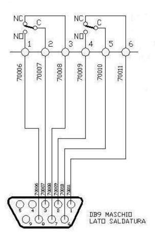
The terminal block the reporting of failures is so configured:
